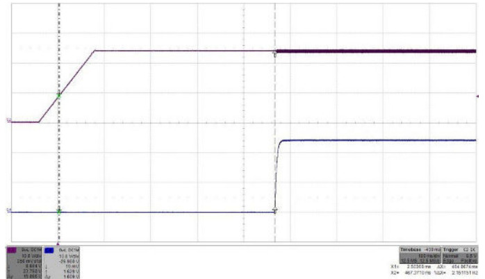
Fig. 23: Turn-on by VIN transient (ON/OFF high) at full rated load current (resistive) at VIN = 24V. Top trace (C2): Input voltage VIN (10 V/div.). Bottom trace (C4): Output voltage (10 V/div.). Time 100 ms/div.
