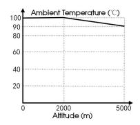
Note: ① With an AC input between 180-200VAC and a DC input between 254-282VDC, the output power must be derated as per temperature derating curves;
