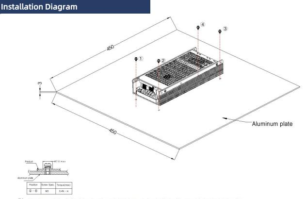
Note: 1. In order to meet the "Derating Curve", the product testing must be installed onto an aluminum plate. The size of the suggested aluminum plate is shown as above. And for optimizing thermal performance, it is necessary to apply thermal grease on the bottom of the product.
