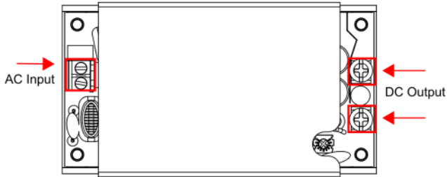
LFM300SXXXC installation diagram
