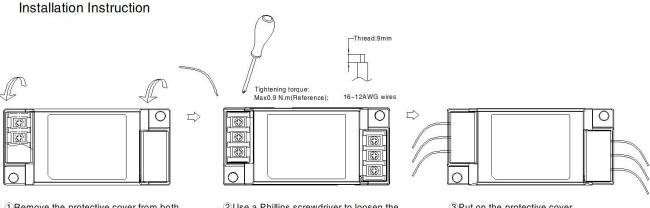
1 Remove the protective cover from both ends to the top;
