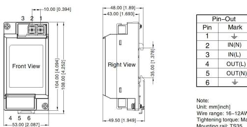
Wire range: 16-12AWG Tightening torque: Max 0.9 N.m Mounting rail: TS35 General tolerances: ±1.00[±0.039]
