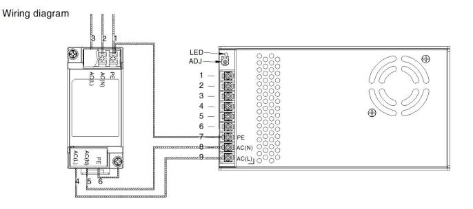
Note: \* The U-shaped ground lug M4 is recommended for PE wire head connection
