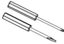
Phillips screwdriver Slotted screwdriver Diameter of the cutting Diameter: 3mm
