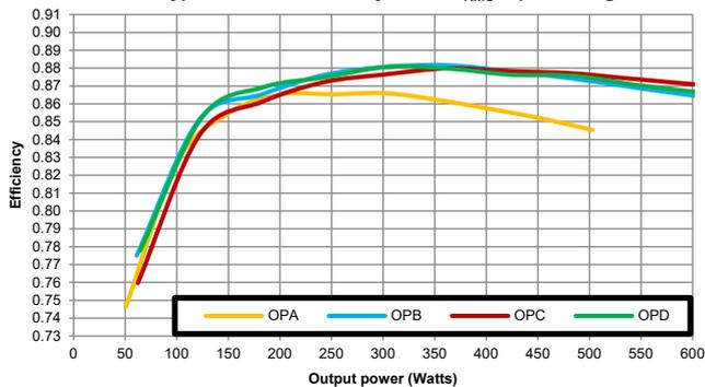
Typical Load Efficiency at 220V<sub>RMS</sub> input voltage
