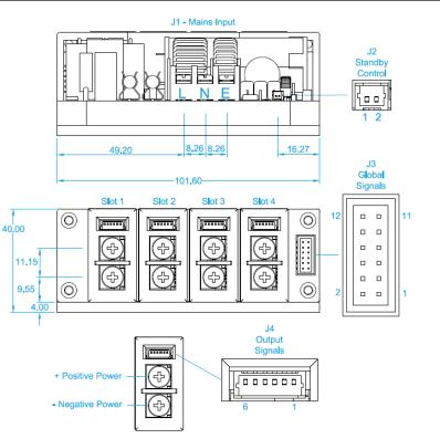
Unless stated otherwise, All dimensions are in milimeters and in accordance with DIN2768-1/-2 CLASS C MATING CONNECTORS
