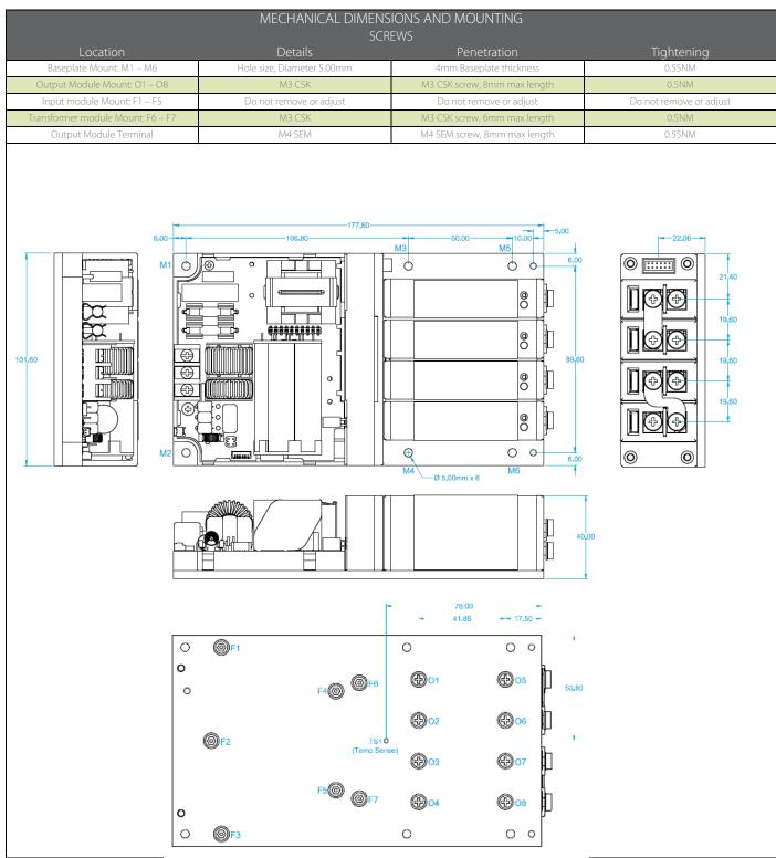
Unless stated otherwise, All dimensions are in millimeters and in accordance with DIN2788-1/-2 CLASS C
