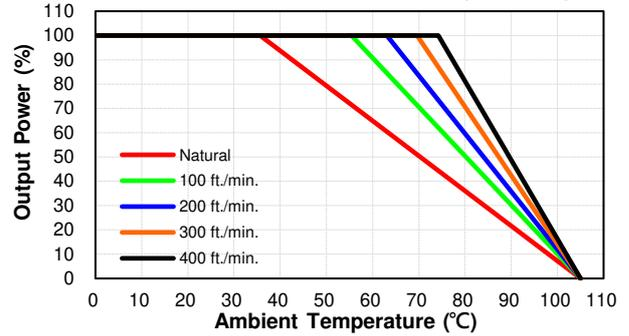
**CQB100W14-72S15, 24, 28, 54 Derating Curve with Heatsink QBT210 (Vin=72V)**
