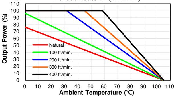
CQB100W14-72S05, 12 Derating Curve with Heatsink QBL127 (Vin=72V)
