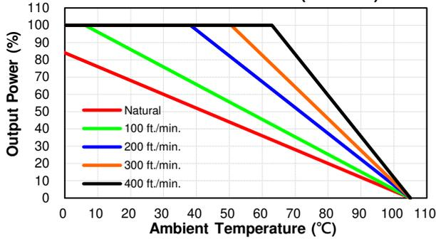
**CQB100W14-72S15, 24, 28, 54 Derating Curve with Heatsink QBL127 (Vin=72V)**
