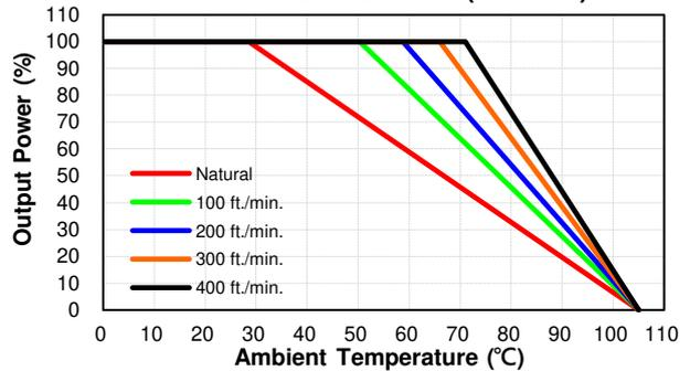
CQB100W14-72S05, 12 Derating Curve with Heatsink QBT210 (Vin=72V)
