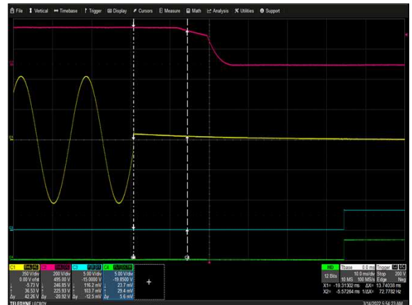
Figure 4: LCM4000HV-T Hold-up Time Vin = 520Vac Load: Io = 16A Ch 1: Vin Ch 2: Vo Ch 3: AC_OK Ch 4: DC_OK
