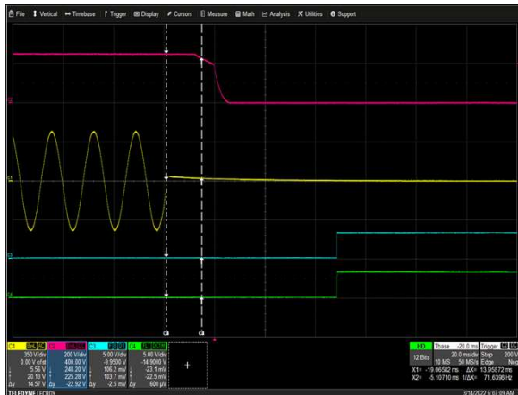
Figure 3: LCM4000HV-T Hold-up Time Vin = 311Vac Load: Io = 16A Ch 1: Vin Ch 2: Vo Ch 3: AC_OK Ch 4: DC_OK
