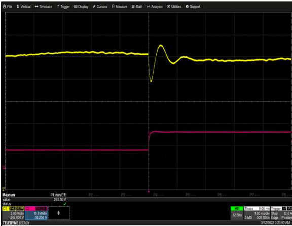
Figure 7: LCM4000HV-T Transient Response - Vo Deviation 50% to 100% load change, 1A/uS slew rate Vin = 380Vac Ch 1: Vo Ch 2: Io
