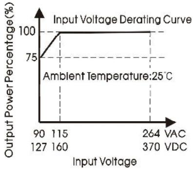
Note: With an AC input voltage between 90 - 115VAC and a DC input between 127 - 160VDC the output power must be derated as per the temperature derating curves
