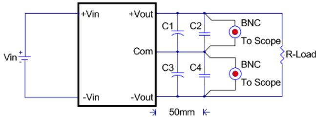
Note: C1 & C3: None, C2 & C4: 1uF ceramic capacitor.
