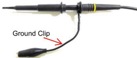
Another method is shown in below, in case of coaxial-cable/BNC is not available. The noise pickup is eliminated by pressing scope probe ground ring directly against the -Vout terminal while the tip contacts the +Vout terminal. This makes the shortest possible connection across the output terminals.
