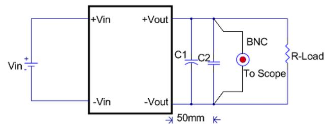
Note: C1: None, C2: 1uF ceramic capacitor.
