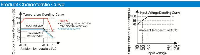
Note: With an AC input voltage between 85-115VAC and a DC input between 120-160VDC the output power must be derated as per the temperature derating curves
