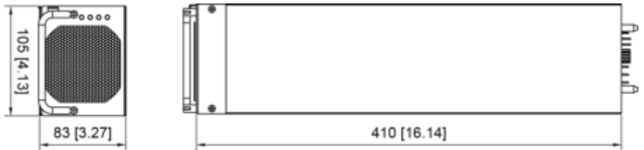
Figure 1. SR-1600 Plus mechanical drawing-single module
