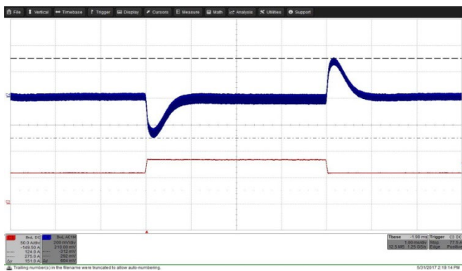
Fig. 29: Output voltage response to load current step change 70% - 100% - 70% (58.5A-84A-58.8A) with di/dt = 0.5A/\mu s at Vin = 14V. Top trace (C4): Output voltage (200 mV/div.). Bottom trace (C3): Load current (50A/div.). Time: 1ms/div.
