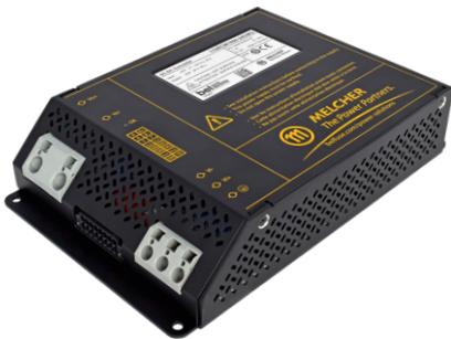
The RCM500 and RCM1000 Series converters are reliable power supplies for railway and transportation systems. They are optimized for 72 or 110 V railway batteries. The output delivers 24 V with 500 or 1000 W. The converters are designed for chassis mounting and exhibit a closed housing with cooling openings.
