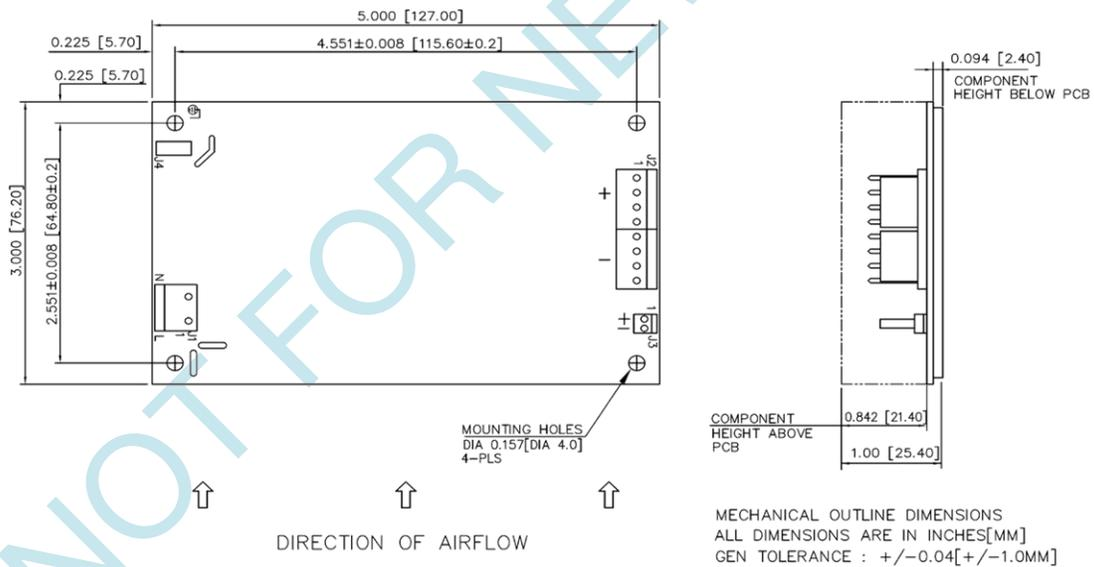
Figure 2. Mechanical Drawing - Molex Header (Option 2)
