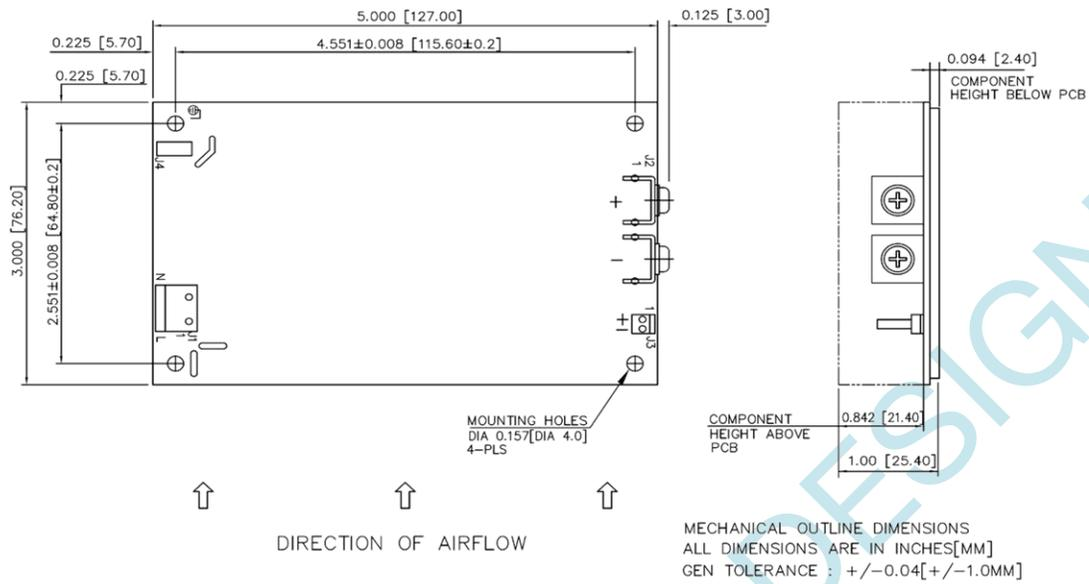
Figure 1. Mechanical Drawing - Screw Terminal (Option 1)
